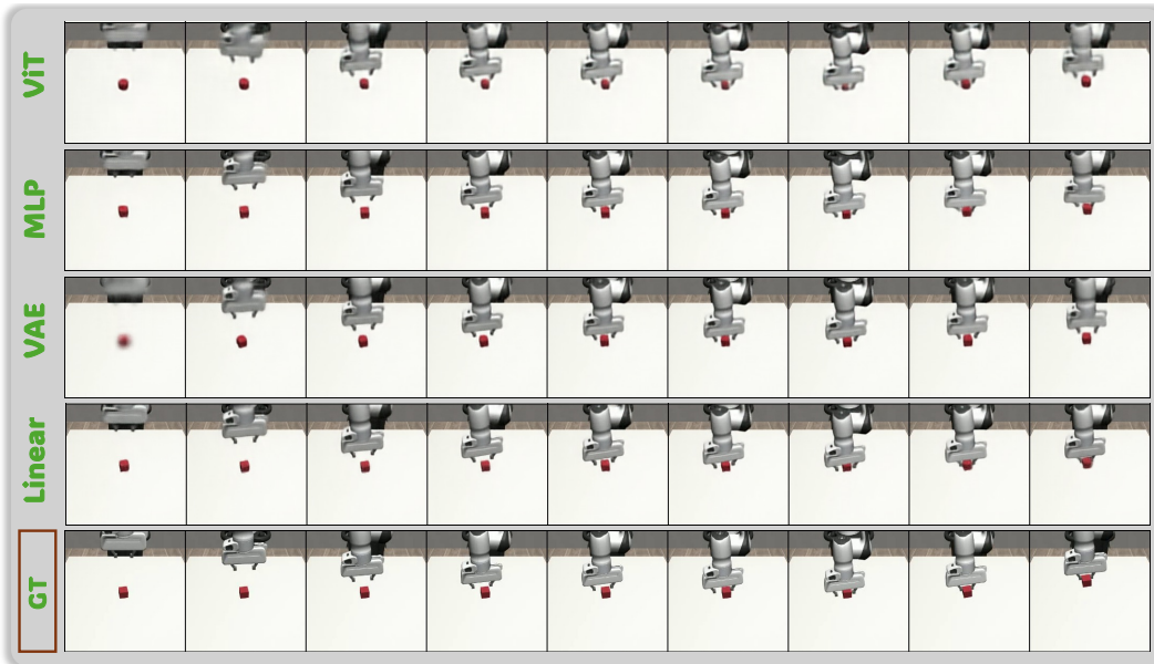
Figure A4: Open-loop rollouts on Lift under different projection architectures (linear vs. MLP / VAE / ViT). The linear projection of TC-WM preserves geometric structure best.
